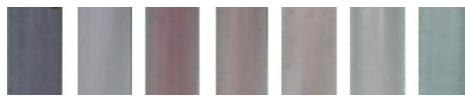
Fig. 2. Photograph of seven samples 1–7 with initial molar ratio 2:1, 3:1, 3.5:1, 5:1, 6.5:1, 8:1 and 9.5:1 of LPEI (repeating unit) to gold (from left to right).
